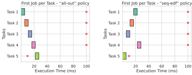
(a) all-out : jobs are launched concurrently. CUDA queues and schedules them in FIFO order. Urgent tasks are not prioritized. (b) seq-edf : jobs are scheduled one at a time in EDF order. Urgent tasks are executed early and meet their deadlines.
