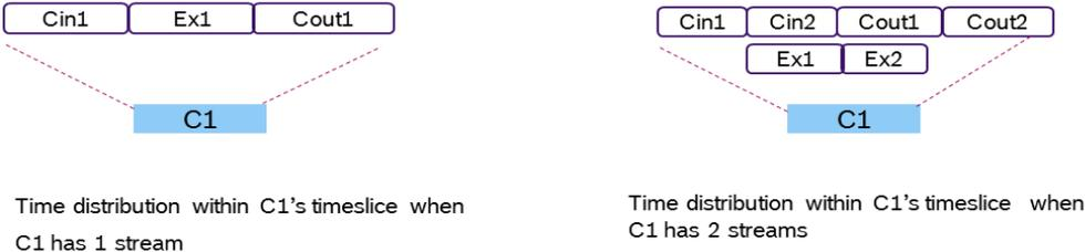
Figure 4: Parallelism with multiple streams
