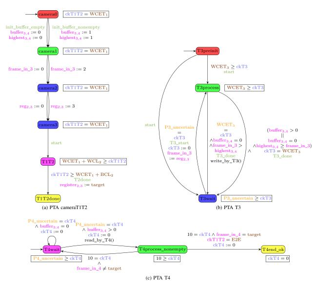
Fig. 1: Modeling the system of Challenge 1A for n = 1
