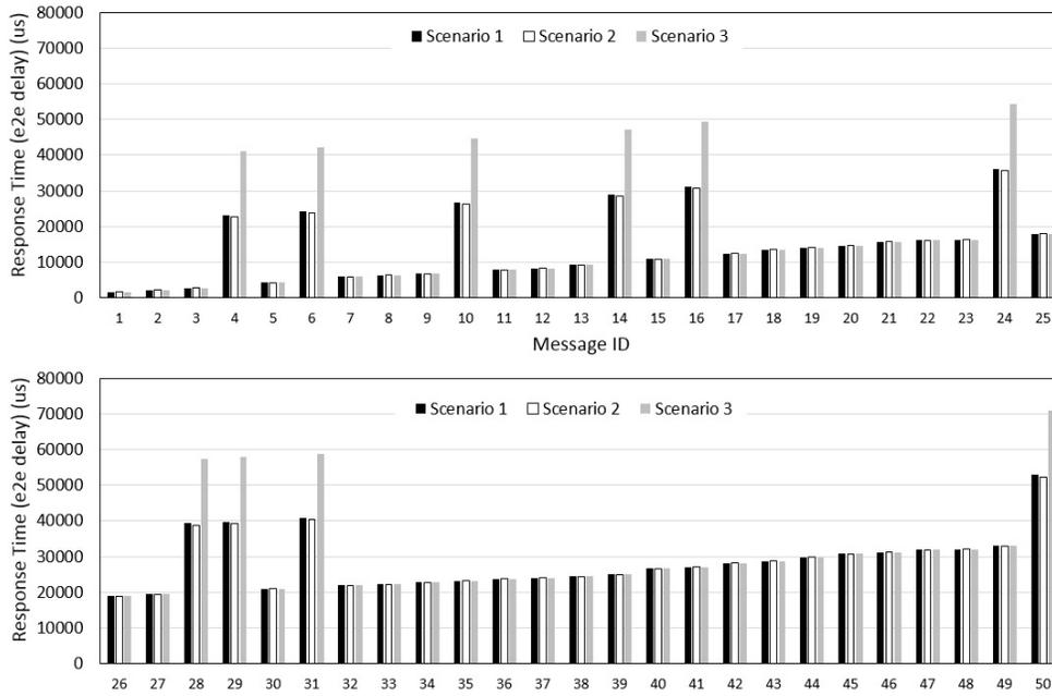
Fig. 5. Response times and end-to-end (e2e) delays of local and global CAN messages respectively.
