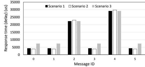
Fig. 6. Response times/delays of Ethernet local/global messages respectively.
